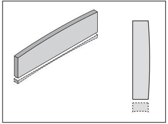
Figure 31. Illustration of edge jointing results.
